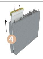
The SISMO-C is removed by means of the extraction tool supplied, leaving a perfect expansion joint between the both walls (EUROCODE 8 compliance).
